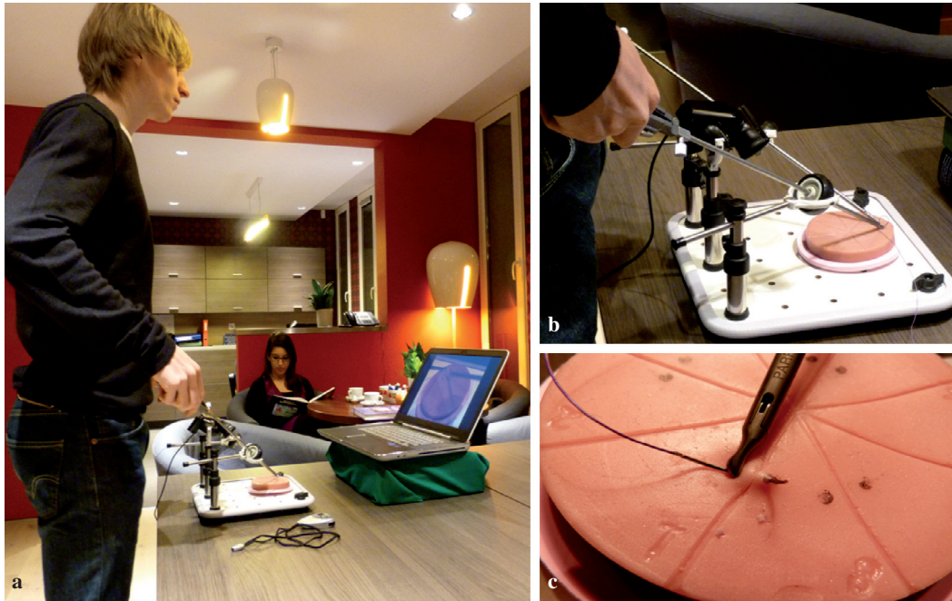
Fig. 4. — “E-Knot “. The easy home trainer a. Student training suturing skills at home. b. E-Knot with camera connected to notebook. c. Suturing pad with 8 different stitching directions.
